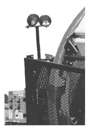
Customer supplies own light brackets mounted on top of side guards. Light package consists of 3 lights and one on/off toggle switch. Usually the lights are mounted with 2 lights facing to the rear and 1 facing to the front.
