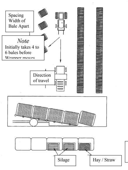
If bales are brought to the site before wrapping, arrange them to allow easy access to bales and allow Wrapper plenty of room to move.
